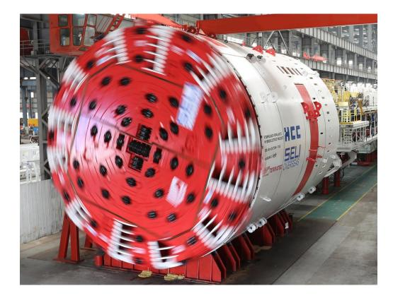
Other state-of-the-art features on the TBM include High-Speed regripping system, Single-Shield advancing mode, High-Pressure Emergency Thrust, Flood Control Doors and many others. The key parts of the TBM were produced in Australia and Japan. The assembly of the TBM was performed at TERRATEC facilities in China.
