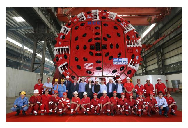
SELI Overseas will execute the Low Pressure Head Race Tunnel in subcontract to HCC (India). The Italian Tunnelling Contractor and TERRATEC have jointly developed the design features of this Ø9.86m Hard Rock Double Shield TBM with which to complete the 13km tunnel, 700m of addit and 12.3km of Main Tunnel.
